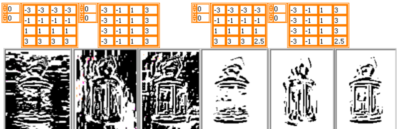
Fig.12. 5x5 Prewitt operator and 5x5 modified Prewitt operator
