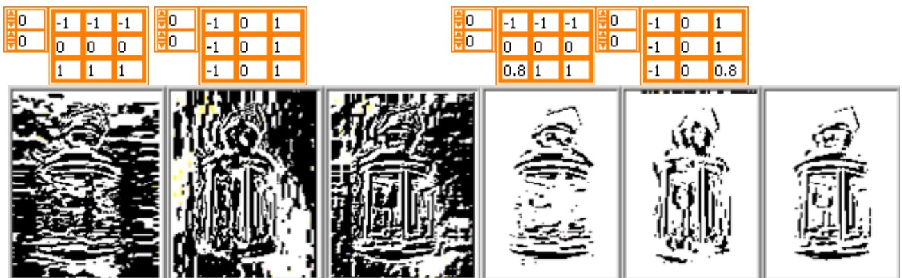
Fig.11. 3x3 Prewitt operator and it's modification
